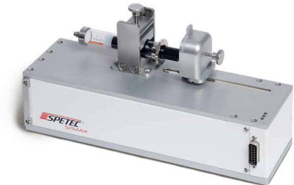
The Spetec syringe pump is used for metering fluids in the microliter and nanoliter range. Its core components consist of the stepper motor drive, high-precision carriage, adjustable syringe holder, and replaceable syringe. Thanks to the high resolution of 25,600 steps per revolution, individual steps during the movement sequence are barely perceptible.
