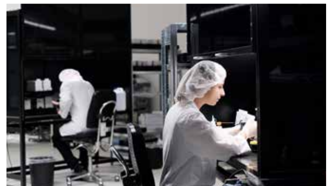
Laminar Flow Boxes in the field: Optics and laser production
